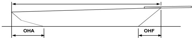
**LWL** = LOA – (OHF + OHA) Include stem and stern posts, exclude rudder. **Beam** = Maximum beam excluding rub rails, etc.
